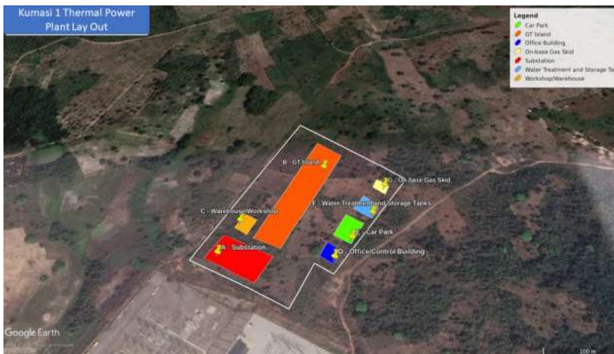
Proposed Layout of Kumasi 1 Thermal Power Plant
