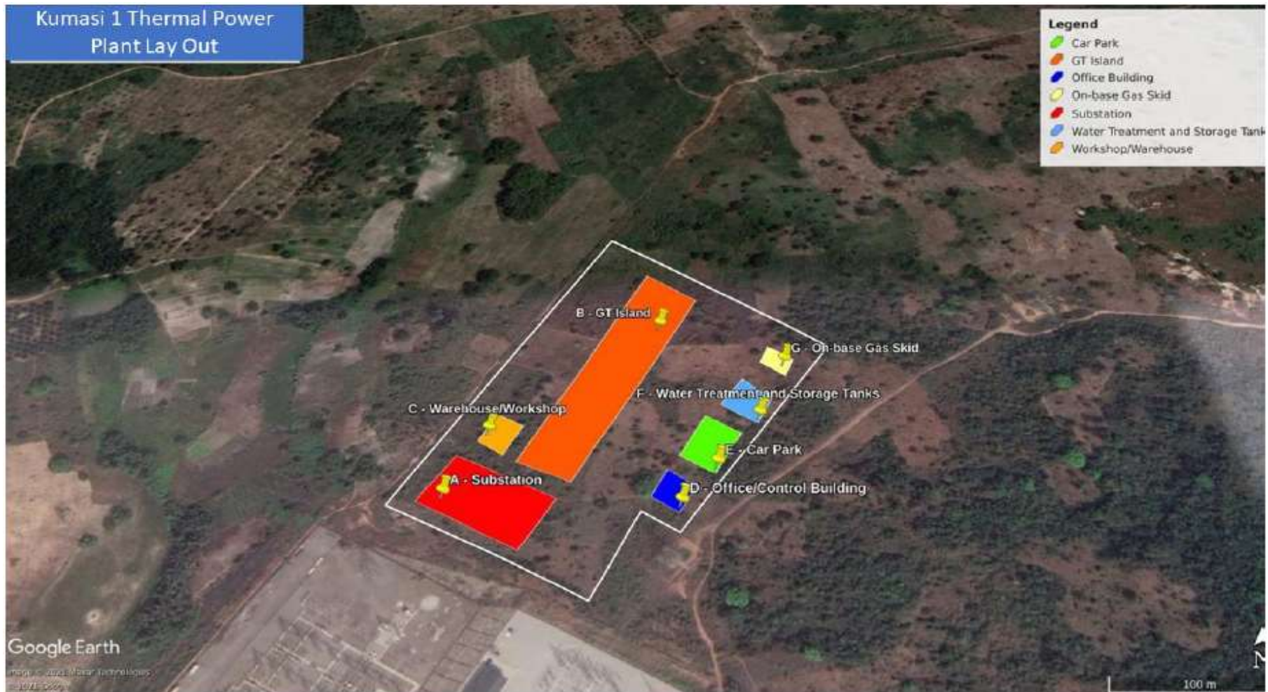
Figure 3-2: The proposed layout of the Kumasi 1 Thermal Power Plant
